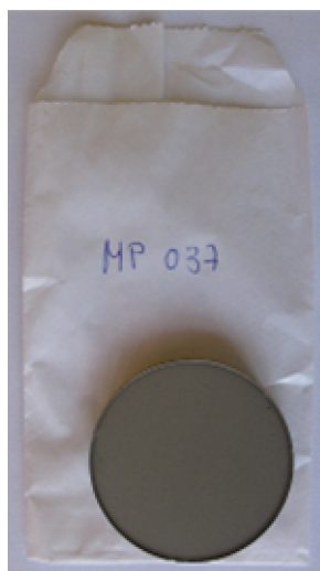
Figure 8: Sediment pastille used for the analysis of trace elements by X-ray fluorescence.
