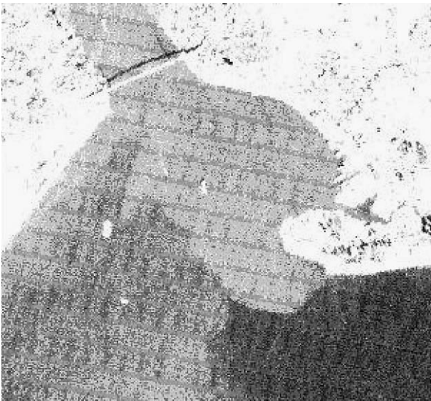
Fig. 4. Landsat TM red (TM3) reflectance south of the Verrazzano Narrows Bridge for 12/27/96 9:20 AM. The image contrast is “stretched” to highlight the variability in the reflectance from water. The regular pattern of near-horizontal lines in reflectance is sensor noise. The image width is 9 km.
